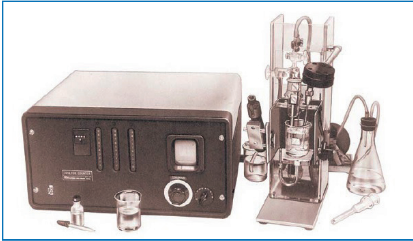
Figure 11. Example of the first automatic blood count device developed by Coulter Brothers (9)
